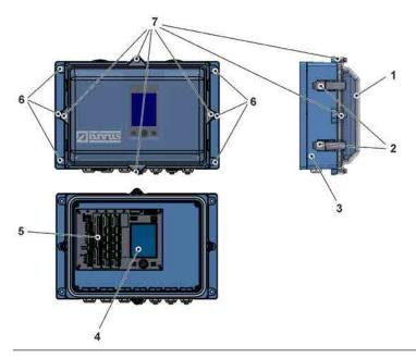
Fig. 20-1 Fastening the field enclosure
