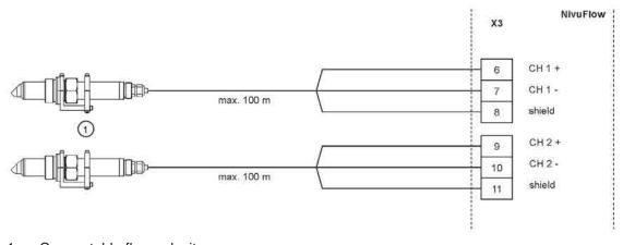
1 Connectable flow velocity sensors
