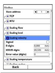
Fig. 34-4 Programming measurement value scaling
