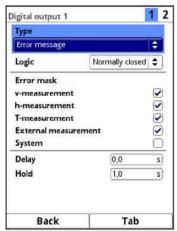
Fig. 31-16 Digital outputs: Activation / Limit contact flow / Error message
