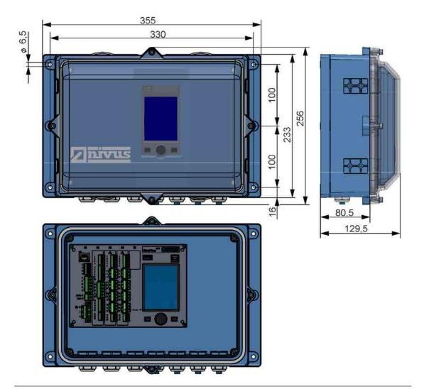
Fig. 15-3 Dimensions of field enclosure NivuFlow
