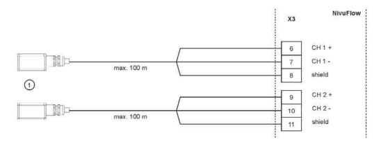
1 Connectable clamp-on sensors
