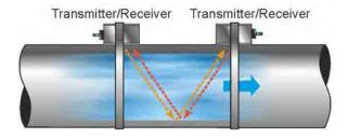
Fig. 22-2 Example "Diametral V" mode
