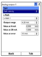
Fig. 31-14 Analog outputs: Activation / Flow / Path velocity
