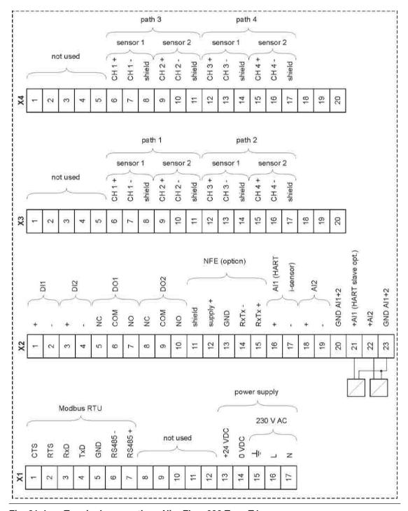
Fig. 21-4 Terminal connections NivuFlow 600 Type T4
