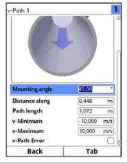
Fig. 28-4 Enter the mounting angle (Clamp-on)
