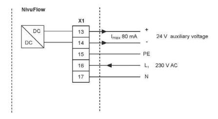
Fig. 21-9 AC power supply wiring
