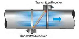
Fig. 22-1 Example "Diametral \" mode
