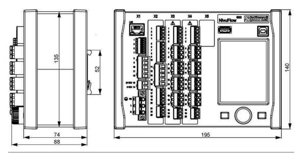
Fig. 15-2 Dimensions of NivuFlow 600 enclosure type E0
