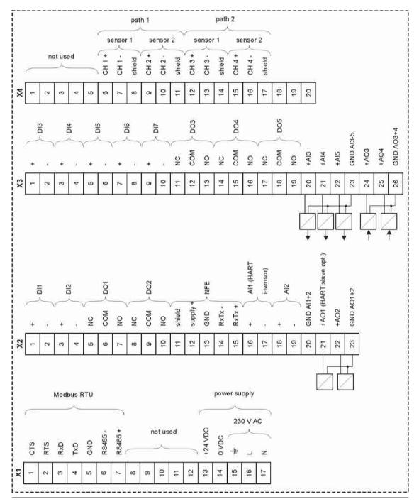
Fig. 21-6 Terminal connections NivuFlow 600 Type TZ
