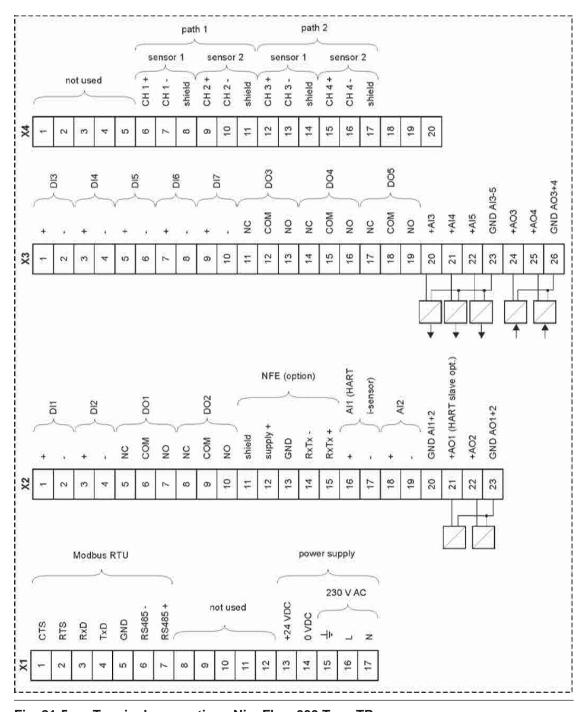
Fig. 21-5 Terminal connections NivuFlow 600 Type TR
