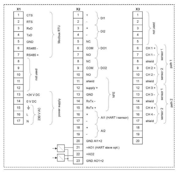
Fig. 21-3 Terminal connections NivuFlow 600 Type TM
