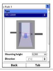
Fig. 31-11 Sensor mounting "Insertion" in pipe or rectangle
