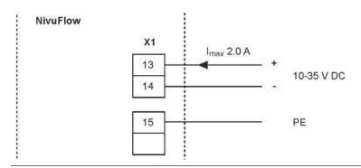
Fig. 21-8 DC connections of power supply
