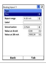
Fig. 31-13 Analog inputs: Activation / Ext. Reading / Flow
