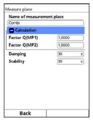
Fig. 31-7 Setting parameters in measurement place Combi menu
