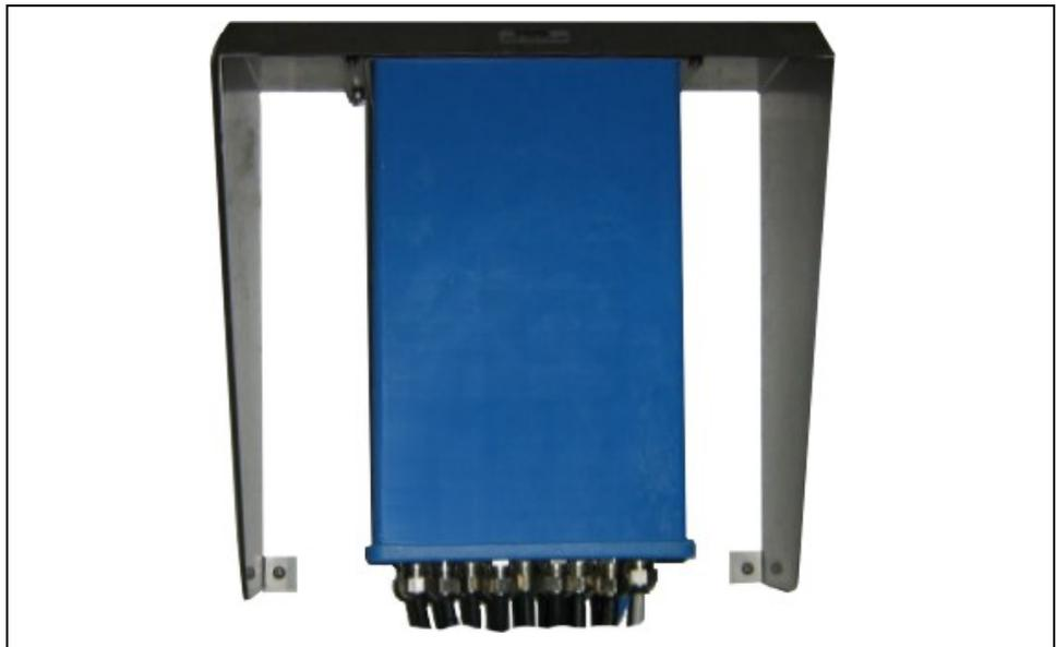
**Fig. 5-27** Suggested installation of adapter box
