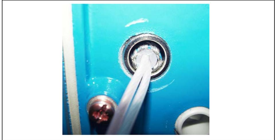
**Fig. 5-23** Inserted sensor cable - inside view
