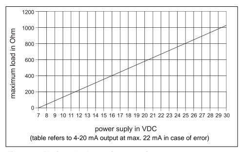
Fig. 6-4 Maximum load at 3- wire connection
