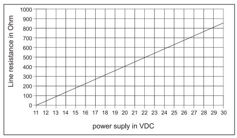
Fig. 6-3 Maximum permissible line resistance at 2- wire connection
