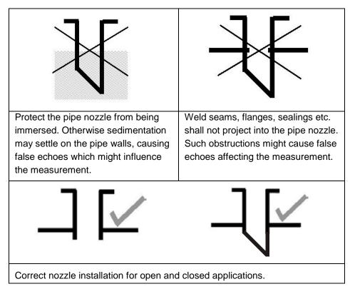
Fig. 6-15 Installation using a pipe nozzle
