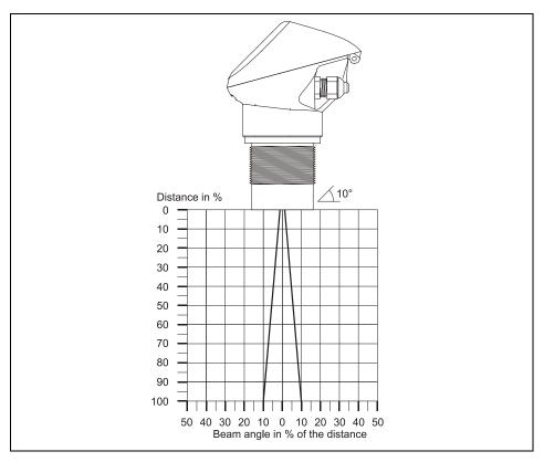
Fig. 6-13 Beam angle
