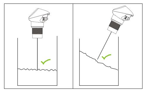
Fig. 6-11 Correct installation of the compact echo sounder
