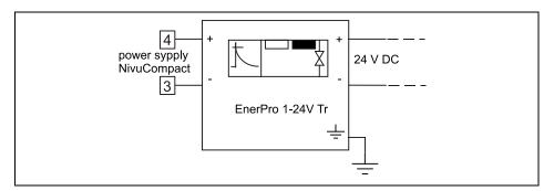
Fig. 6-10 Overvoltage Protection of operation voltage supply (only 3/4-wire operation)
