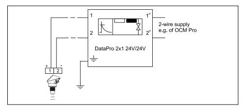
Fig. 6-8 Overvoltage Protection of 2-wire supply
