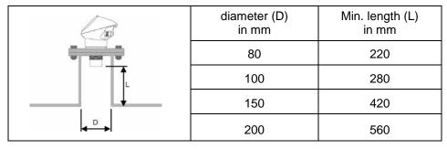
Fig. 6-14 Dome top on pipe measuring section: installation dimensions
