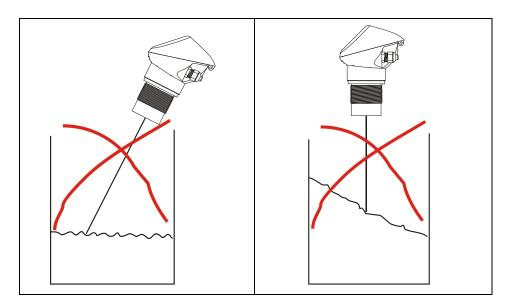
Fig. 6-12 Incorrect installation of the compact echo sounder
