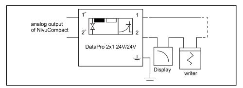
Fig. 6-9 Overvoltage Protection of analog Outputs
