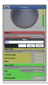
Fig. 36-12 Programming integrated pressure sensor
