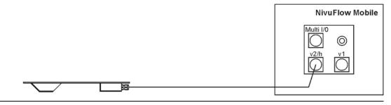
Fig. 25-2 Connection of level sensor DSM-L0
