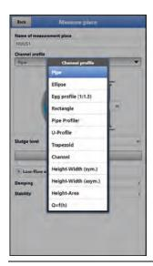
Fig. 36-2 Selectable channel profiles
