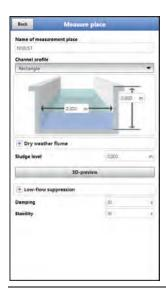
Fig. 36-3 Example of a channel profile menu
