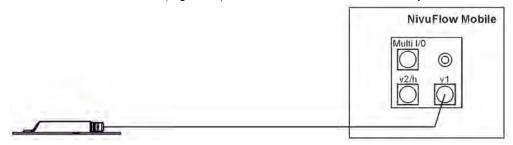
Fig. 25-1 Connection of flow velocity sensor CSM, CSP and NPP
