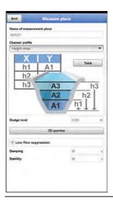
Fig. 36-4 Setting of profile using height-width (sym.)
