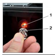
Fig. 31-20 Waking up the NivuFlow Mobile
