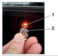
Fig. 31-10 Waking up the NivuFlow Mobile
