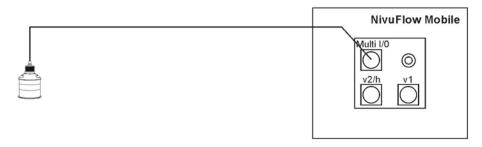
Fig. 25-3 Connection of level sensor i-Series and NivuBar Plus
