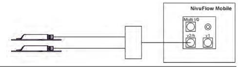
Fig. 25-4 Connecting two flow velocity sensors via the Adapter Box
