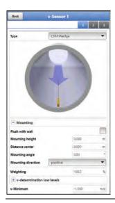
Fig. 36-14 Programming using height, distance and angle
