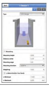
Fig. 36-18 Entering sensor position, in relation to the application centre
