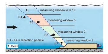
Fig. 21-1 Situation at first signal detection
