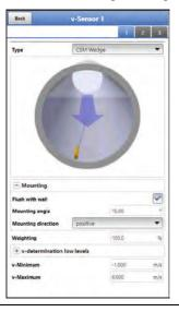
Fig. 36-15 Parameter setting only by entering the angle
