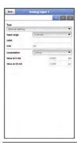
Fig. 36-24 Analog input as external reading
