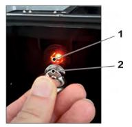
Fig. 31-1 Waking up the NivuFlow Mobile
