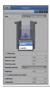
Fig. 36-19 Modifying the sensor mounting direction
