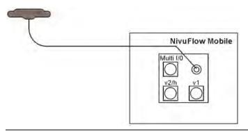
Fig. 28-1 Connection GPRS Antenna
