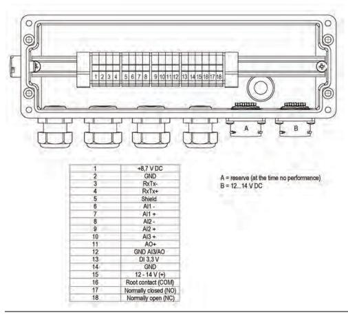
Fig. 27-2 Connector Box terminal wiring
