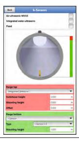
Fig. 36-10 Indication of programmable ranges
