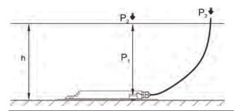
Fig. 21-7 Determined filling level
