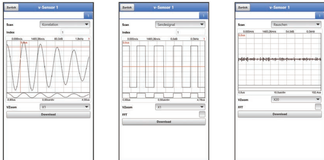
Abb. 39-2 Signalanalyse Korrelation / Sendesignal / Rauschen
