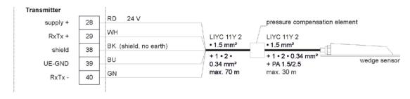
Fig. 14-5 KDA combi sensor with integrated pressure measurement cell, Type KP (Non-Ex)
