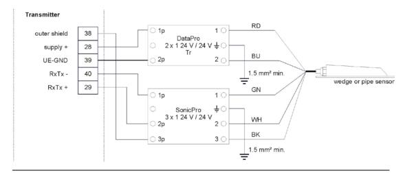
Fig. 14-16 Overvoltage protection for KDA velocity sensor Non-Ex version
