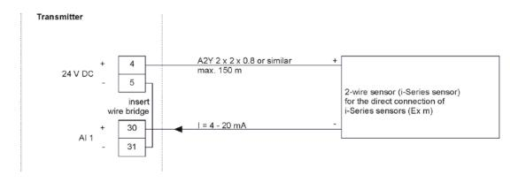
Fig. 14-9 NIVUS i-Series sensor for level measurement in Ex-Zone 1
