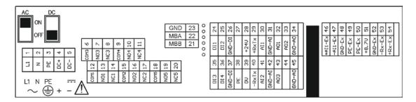
Fig. 14-2 Terminal housing, Ex version
