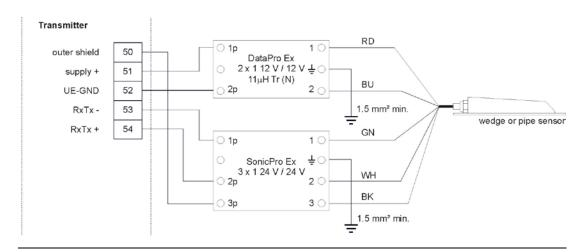
Fig. 14-17 Overvoltage protection for KDA velocity sensor Ex version
