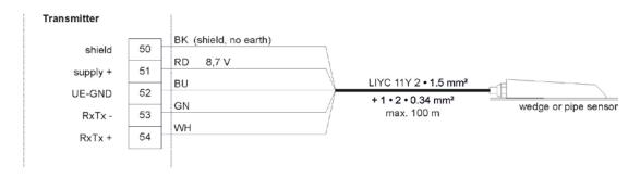
Fig. 14-6 KDA wedge or pipe sensor, Type K0 or R0 (Ex)
