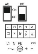
Fig. 14-12 Slide switch position in terminal clamp housing
