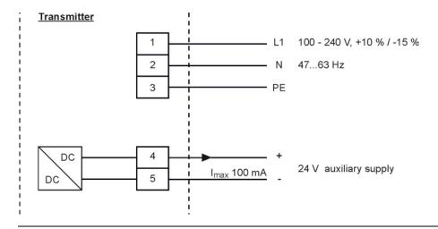
Fig. 14-13 AC model power supply
