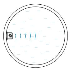
Fig. 23-14 Sensor type 2: Constant level
