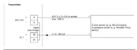
Fig. 14-8 Ext. 2-wire sensor for flow level measurement (Non-Ex)
