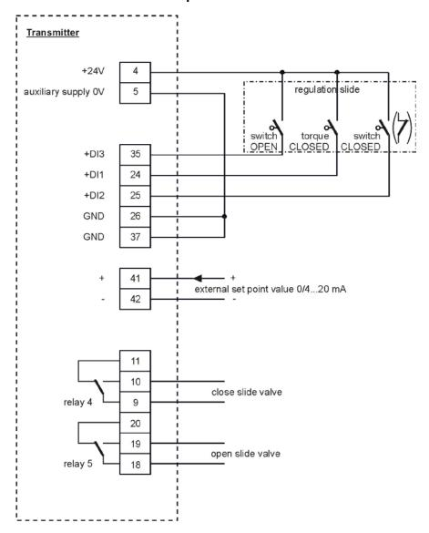
Note: Relay 1, 2 and 3 are not suitable to control the regulation slide valve.
