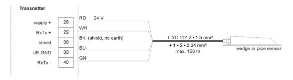
Fig. 14-4 KDA wedge or pipe sensor, Type K0 or R0 (Non-Ex)
