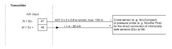
Fig. 14-10 Ext. 2-wire sensor for level measurement (Ex)
