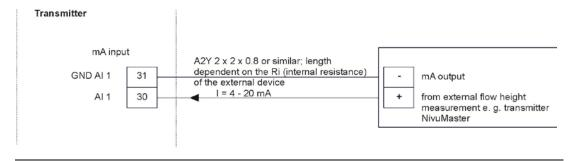
Fig. 14-11 Ext. flow level measurement via NivuMaster
