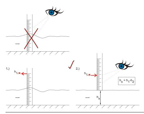
Fig. 27-1 Determination of reference level under operating conditions
