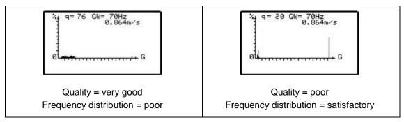
Fig. 24-9 Flow velocity profiles
