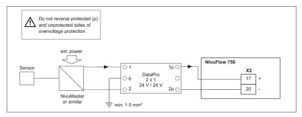
Fig. 5-21 Overvoltage protection of 4-20 mA input from external transmitter
