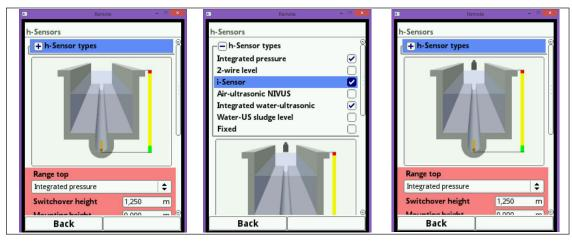
Fig. 7-28 Sensor selection and indication of sensor measuring ranges
