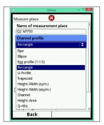
Fig. 7-8 Selectable channel profiles
