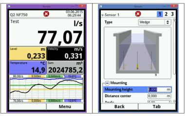
Fig. 8-16 Settings and positions of flow velocity sensors
