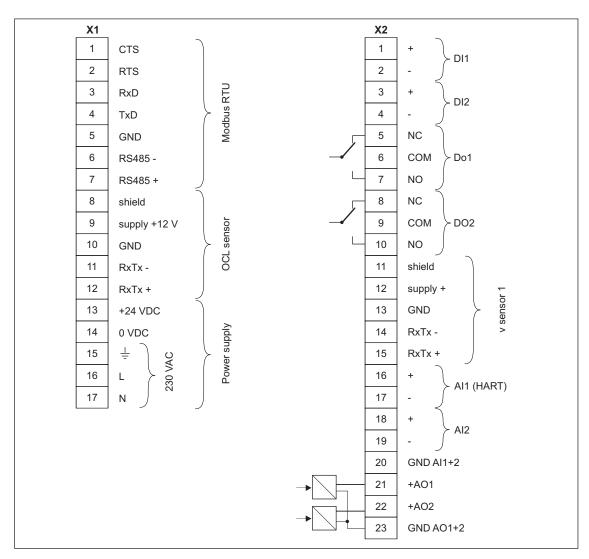
Fig. 5-24 General connection diagram - NivuFlow 750, type S1
