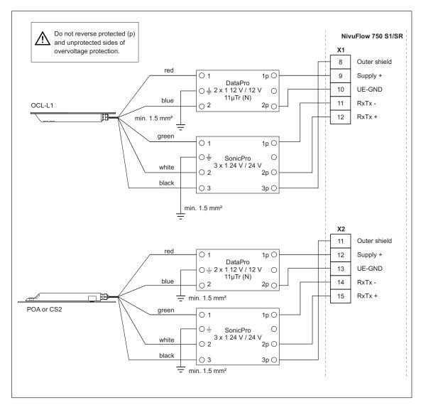
Fig. 5-17 Sensor overvoltage protection for S1/SR
