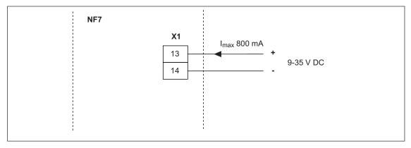
Fig. 5-29 DC connections of power supply
