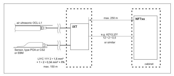
Fig. 5-8 Connecting iXT to NivuFlow via telecommunications cable
