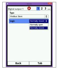
Fig. 7-71 Adjustment options Logic
