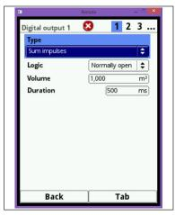
Fig. 7-68 Programming pulse generator
