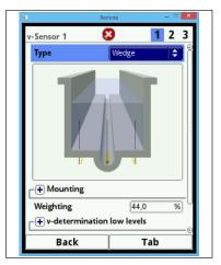
Fig. 7-35 v-Sensor selection transmitter type M3
