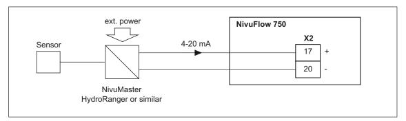
Fig. 5-14 Connecting an external transmitter
