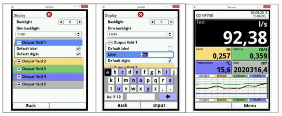
Fig. 8-7 Change text for measurement value
