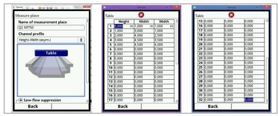
Fig. 7-21 Setting parameters using free asymmetric height-width-width profile
