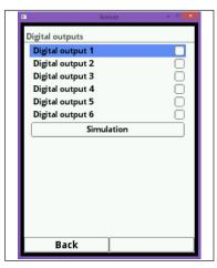
Fig. 7-101 Display status of digital outputs
