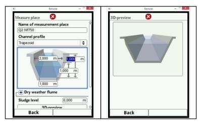
Fig. 7-17 Programming trapezoid profile without rectangular top
