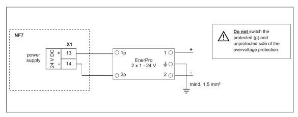
Fig. 5-16 Overvoltage protection for power supply DC
