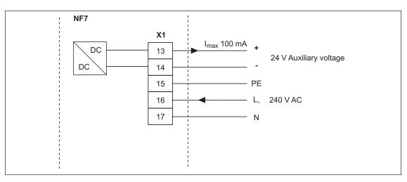
Fig. 5-28 230 V AC connections of power supply
