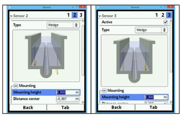
Fig. 7-43 Height position of v-sensor 2 and 3 are set correctly
