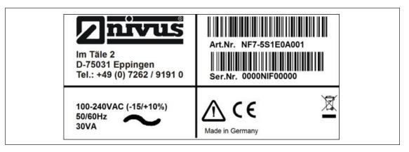
Fig. 3-3 Nameplate AC version
