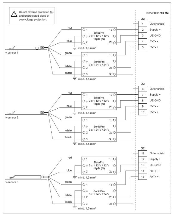
Fig. 5-19 Overvoltage protection Flow velocity sensor to M3
