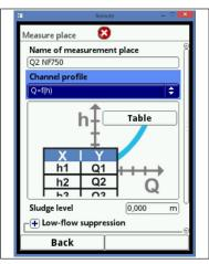
Fig. 7-23 Programming Q/h-characteristics
