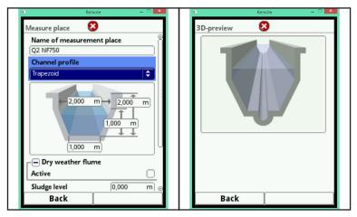
Fig. 7-16 Programming trapezoid profile with rectangular top
