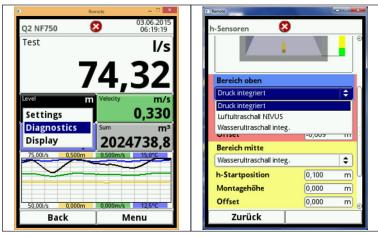
Fig. 8-11 Direct selection of individual sensor diagnostics
