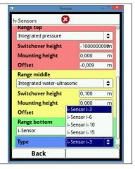
Fig. 7-32 Programming i-Sensor type
