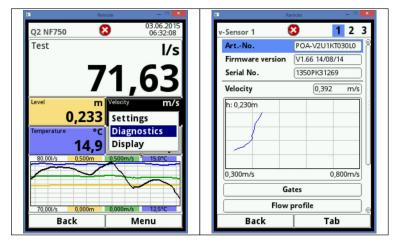
Fig. 8-17 Information on the flow velocity sensor
