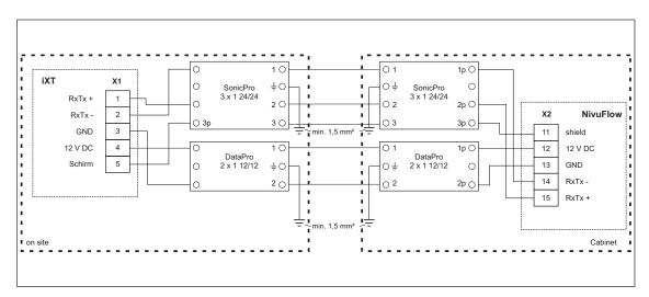
Fig. 5-23 Overvoltage protection iXT to NivuFlow 750 S1/SR
