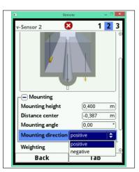
Fig. 7-45 Modifying the sensor mounting direction
