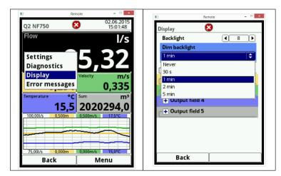
Fig. 8-6 Adjust dimming
