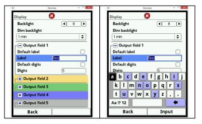
Fig. 7-170 Entering the output field label
