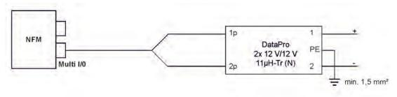
Fig. 25-3 General overvoltage protection for DC power supply
