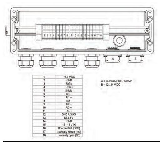
Fig. 27-2 Connector box terminal wiring
