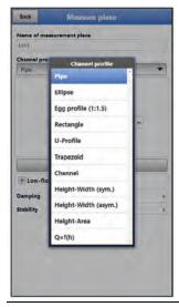
Fig. 38-2 Selectable channel profiles
