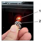
Fig. 31-10 Waking up the NivuFlow Mobile
