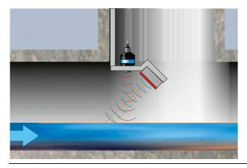
Fig. 21-1 Metering with surface radar
