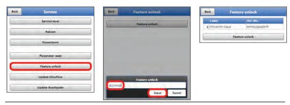
Fig. 40-10 Licence activation in NFM display tool
