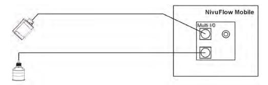
Fig. 25-1 Connection of Radar sensor and i-Series sensor
