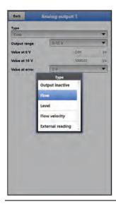
Fig. 38-12 Analog output activation
