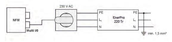
Fig. 25-2 General overvoltage protection for AC power supply
