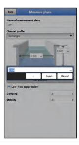
Fig. 33-1 Selecting the channel profile / specifying dimensions
