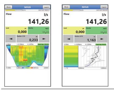
Fig. 28-10 Flow profile from the front and side
