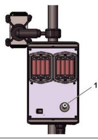
Fig. 25-1 LED on the front of the NivuFlow Stick
