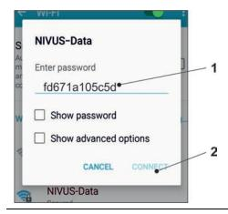
Fig. 26-4 Enter password (here fd671a105c5d as example) and connect
