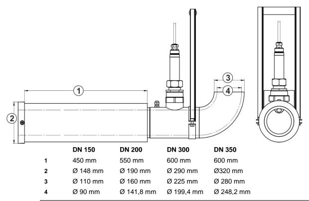
Fig. 4-2 Dimensions NPP0 DN... with built-in pipe sensor POA-V200RT...SG
