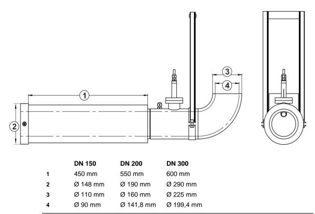
Fig. 4-5 Dimensions NPP0 DN...V2 with built-in pipe sensor CSM-V100RNE15R
