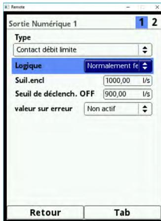
Fig. 23-31 Programmation contact limite
