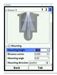
Fig. 23-20 Setting the Mounting Height
