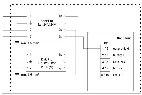
Fig. 17-13 Overvoltage protection iXT to NivuFlow 7550
