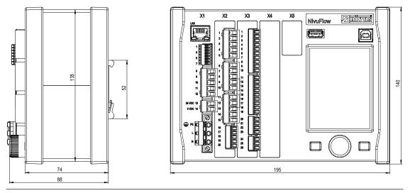
Fig. 9-2 Dimensions of the transmitter NivuFlow 7550
