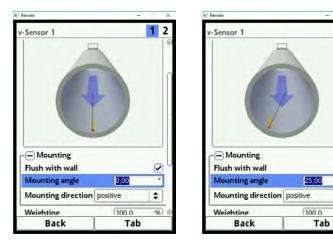
Fig. 23-19 Setting the Mounting Angle Parameter
