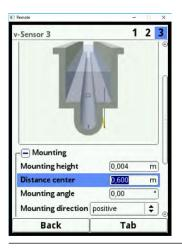
Fig. 23-21 Mounting height of v-Sensor too low
