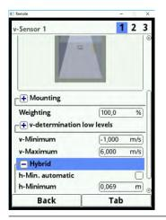
Fig. 23-30 Hybrid for correlation sensor
