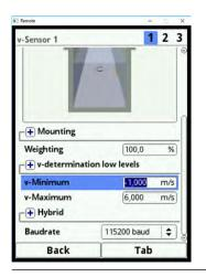
Fig. 23-29 Limiting the velocity evaluation
