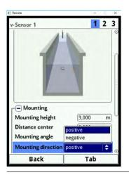
Fig. 23-24 Sensor installation direction altering options
