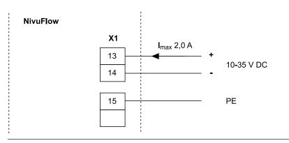
Fig. 18-4 DC connections of power supply
