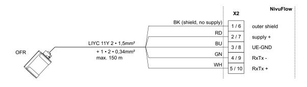
Fig. 17-5 Connection radar sensor, type OFR
