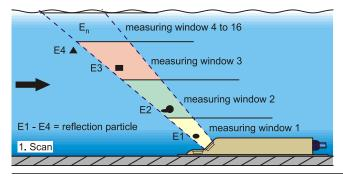
Fig. 13-2 Situation at first signal detection
