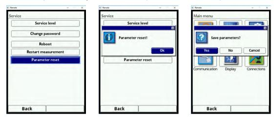
Fig. 25-11 Resetting the parameters to default settings
