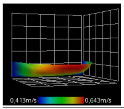
Fig. 13-6 Computed 3-dimensional flow profile
