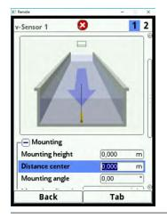
Fig. 23-23 Entering sensor positions related to application centre
