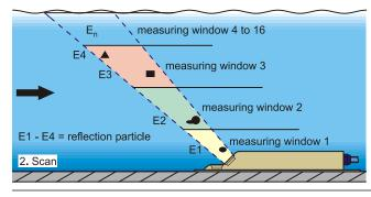
Fig. 13-3 Situation at second signal detection
