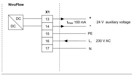
Fig. 18-3 230 V AC connections of power supply
