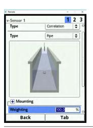
Fig. 23-27 Weighting of v-Sensors
