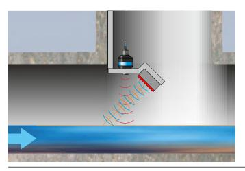
Fig. 13-1 Measurement using Surface Radar
