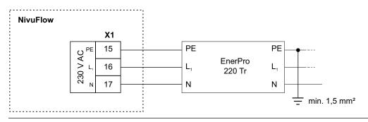
Fig. 17-8 Overvoltage protection for power supply AC
