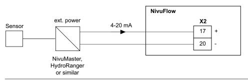
Fig. 17-7 Connecting an external transmitter
