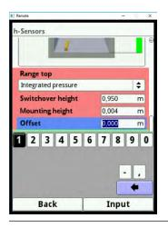
Fig. 23-13 Programming the integrated pressure sensor
