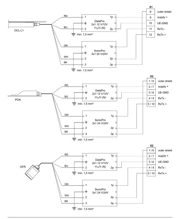
Fig. 17-10 Sensor overvoltage protection for KR1
