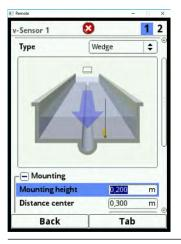
Fig. 23-22 Correct Mounting Height v-Sensor
