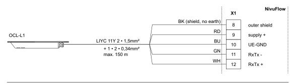
Fig. 17-3 Connection air ultrasonic sensor, type OCL-L1
