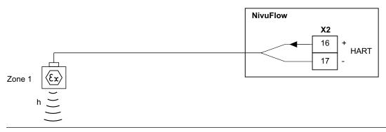
Fig. 17-6 Connecting a 2-wire sensor EX for level measurement
