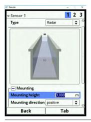
Fig. 23-25 Setting the mounting height
