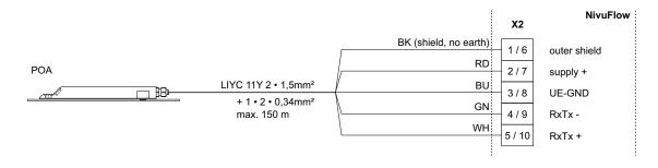
Fig. 17-4 Connection cross correlation sensor, type POA
