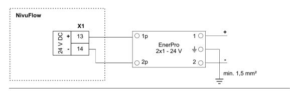
Fig. 17-9 Overvoltage protection for power supply DC
