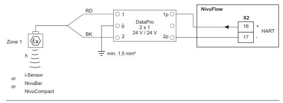
Fig. 17-11 Overvoltage protection external level measurement
